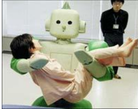
RI-MAN robot is equipped with sensors that show a body's weight, position smell!
